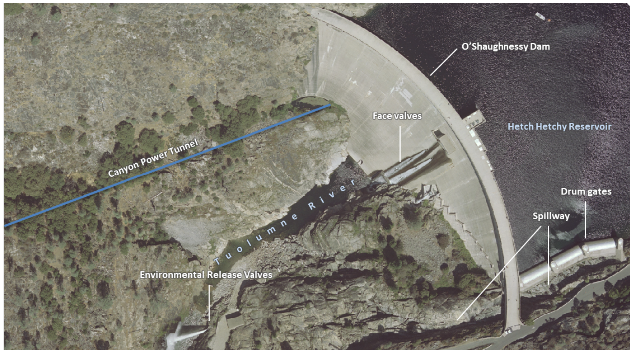
Figure 8. Aerial view of O’Shaughnessy Dam water diversion and release facilities.
